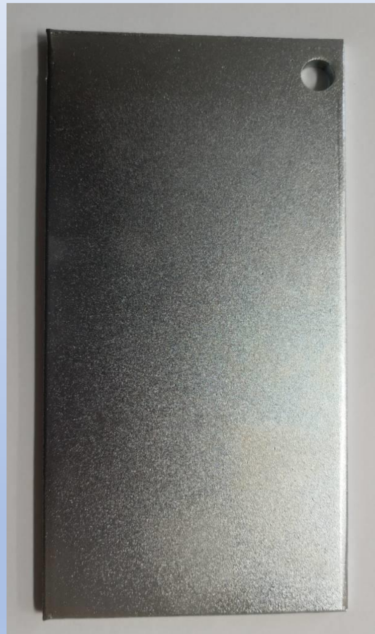
GALVANIZED Zn 15.5 microns
