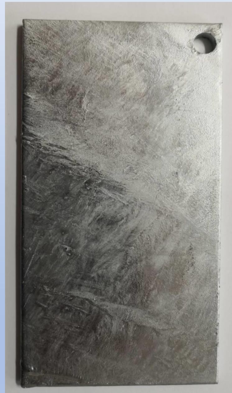
HOT DIP GALVANIZED Zn 73 microns
